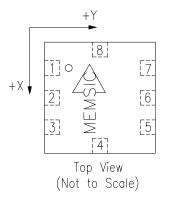
**Note:** The MEMSIC logo's arrow indicates the -X sensing direction of the device. The +Y sensing direction is rotated  $90^{\circ}$  away from the +X direction following the right-hand rule. Small circle indicates pin one(1).
