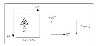
Figure 2: Accelerometer Position Relative to Gravity
